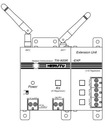
TW-800R-EXP ×1 (Dipole antenna for ANT2 is set at shipment) ※ANT2 is fixed by resin before shipment by regulation of FCC/IC in an applicable country.
