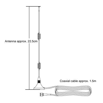
\*ANT2 is fixed by resin before shipment by regulation of FCC/IC in an applicable country.
